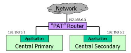
For example, if Central node #1 has IP address 192.168.5.1 and node #2 has IP address 192.168.5.2, a router can be configured to overload IP address 192.168.6.3. 192.168.6.3 would be the only IP address the rest of the world would know about; neither of the 192.168.5.\* addresses would need to be configured in any IP-specific firewall or configuration.
