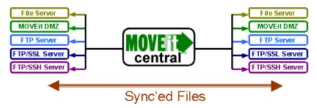
Folder sync operations are configured in special "synchronization tasks". Instead of the sources and destinations found in a traditional task, a synchronization task consists of "Folder A", "Folder B" and a "sync direction" arrow. Possible sync directions include "one-way" and "two-way", and there are additional options that control whether or not certain deletions or extra files are permitted.
