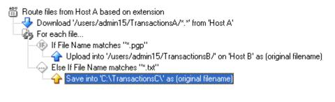
You can create an Advanced Task by opening the Tasks tab, clicking Add Task, and then selecting the Advanced Task type.
