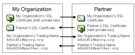
Each AS1, AS2 or AS3 protocol will also require each side to agree on additional protocol-specific items such as which server to send files too, what credentials to use to authenticate to the server and what flavors of MDNs are supported. Additional information about these specifics is covered in each ASx protocol's discussion.
