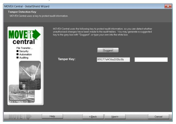
Tamper Key - Enter an arbitrary string into the white box or click Suggest to have the install suggest a random key. If you are installing a failover pair, you must use the same tamper detection key on both machines.
