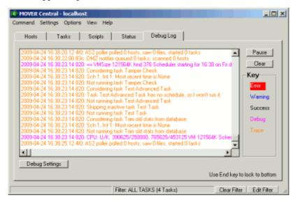
The main screen of MOVEit Central Admin is broken into five or six tabs. Three are used to configure MOVEit Central and two are used to monitor MOVEit Central. One tab ("Failover") only appears if *MOVEit Central Failover* (on page 56) has been licensed.
